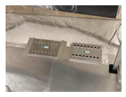
7. Connect antennas to BNC feedthrough, drape cords over absorbers. Connect camera to ethernet feedthrough if
