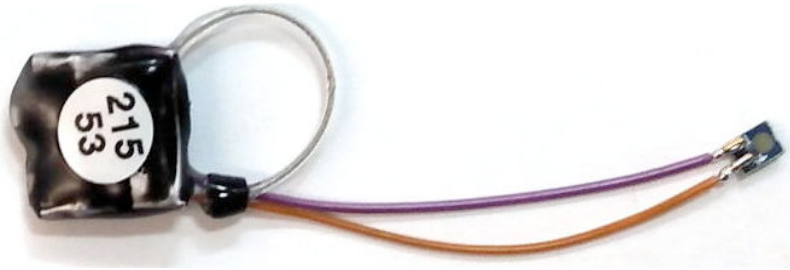
Figure: The Implantable Stimulator-Transponder (A3036C). Volume 0.75 ml, mass 1.3 g, battery capacity 10 mAhr. With a blue FCLED, provides 1-ms flashes of 5 mW blue light at 10 Hz for 67 hours. Sleep life is 1400 hrs. Shown with dummy-lamp that prevents short-circuit of stimulus leads and allows testing before implantation. Recharges through lamp leads in the same way as the MS-ISL.
