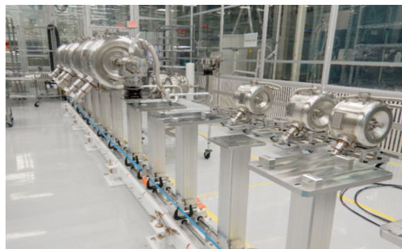
Figure 1: Example Clean-Room Environment, Superconducting Radio-Frequency (SRF) Assembly Room at Fermi National Laboratory (FNL). Courtesy of Mattia Parise, FNL.
