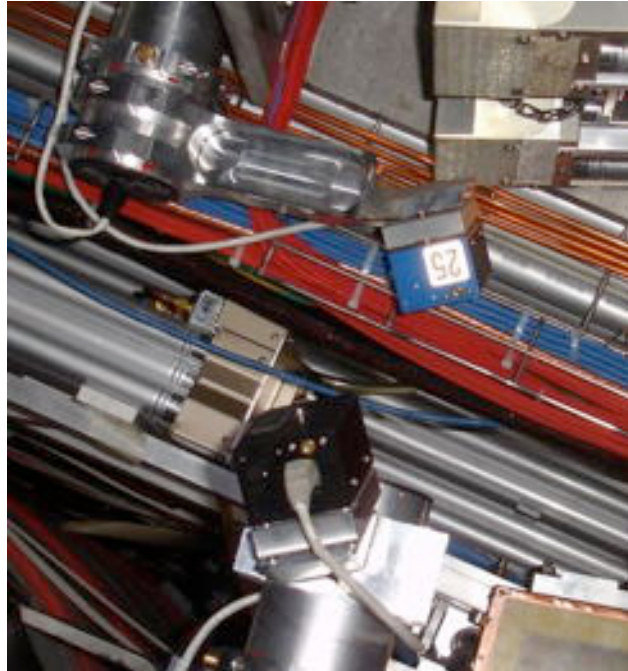
Figure 7: P-BCAMs Manufactured by Brandeis University and Installed in the ATLAS End-Cap Alignment System [9]. Each BCAM is mounted upon a surveyed reference bar.
