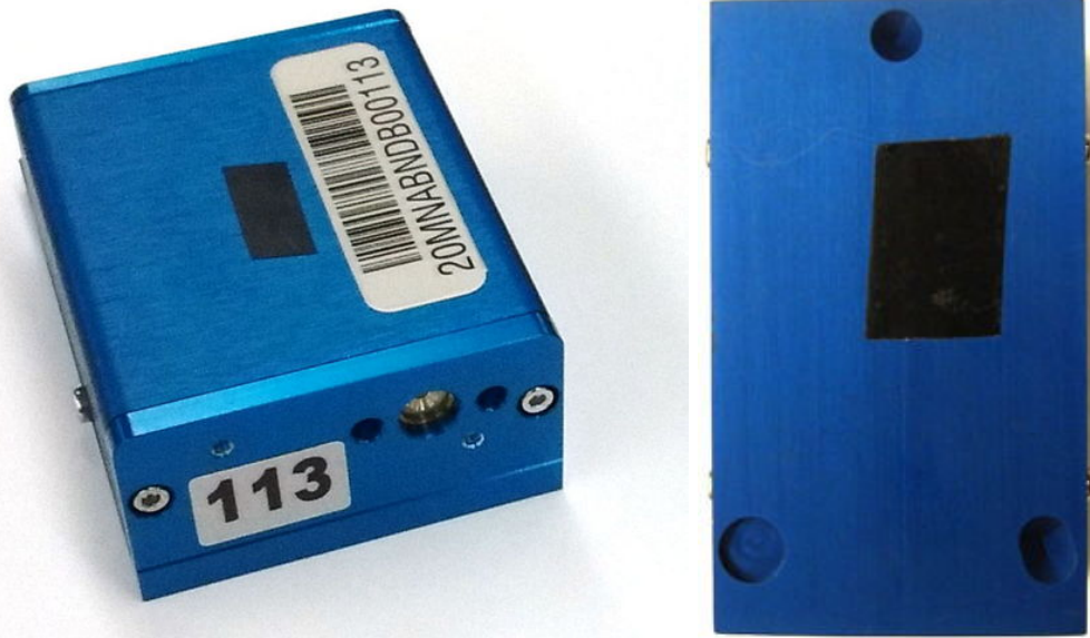
Figure 12: The N-BCAM Used in the ATLAS End-Cap Muon Alignment System. Left: Lens and laser openings visible. Right: Cone, slot, and flat kinematic mounting depressions. The SCAM will look much the same, but without the lasers.
