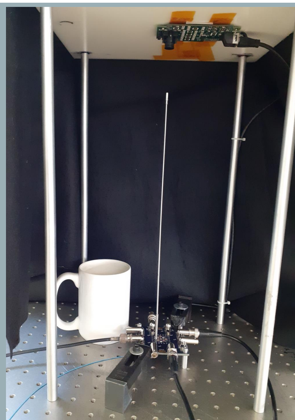
Figure 6: Single fiber positioner surrounded by dark fabric
