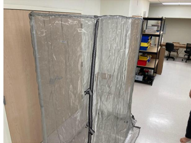
4. Drill through both layers of the magnet strip with a self tapping screw at the top left corner of the metal frame. Drill through only the back layer of the magnet strip at the other corners. The top layer of the magnet strip should only be adhered to the frame at one point. Drill screws into the frame on the rear as shown on next slide.
