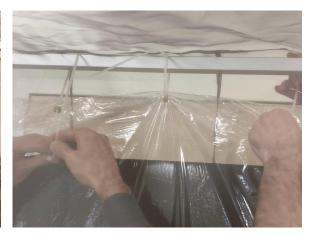
6. Place feedthroughs under the canopy on the back so that half of the board is inside the canopy and half is outside. Tape them down.
