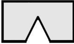
Figure 49: Cut a wedge into the fiber patch
