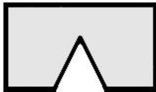
Figure 37: Cut a wedge into the fiber patch
