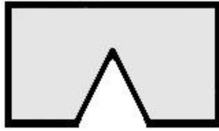
Figure 53: Cut a wedge into the fiber patch
