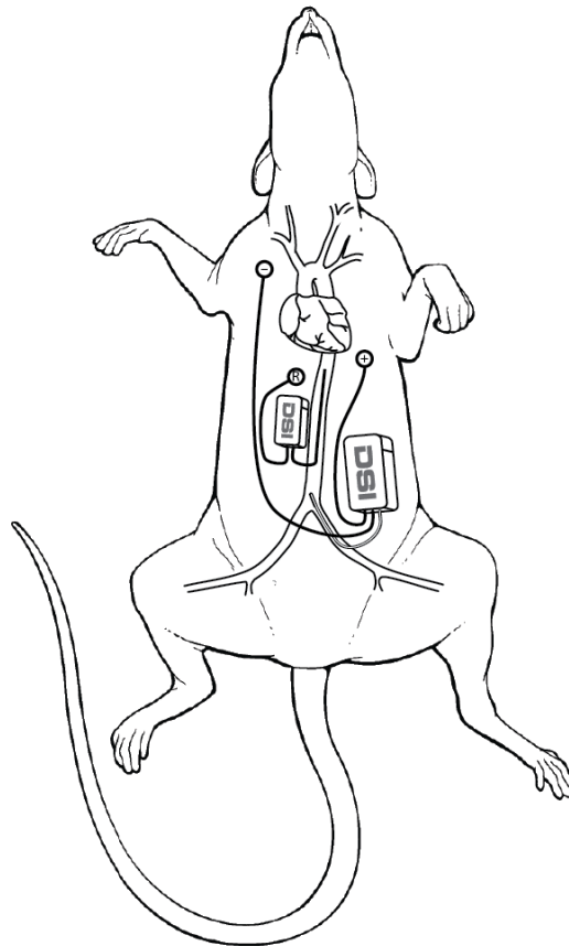
Figure 70: HD-XG device in intra-peritoneally, HD-S11 device subcutaneously on animal's left flank
