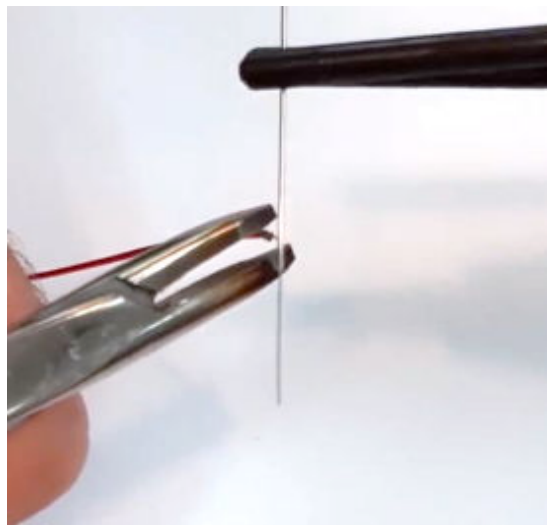
Video: X-Electrode and B-Lead Crimp Connection with Q- Ferrule.
