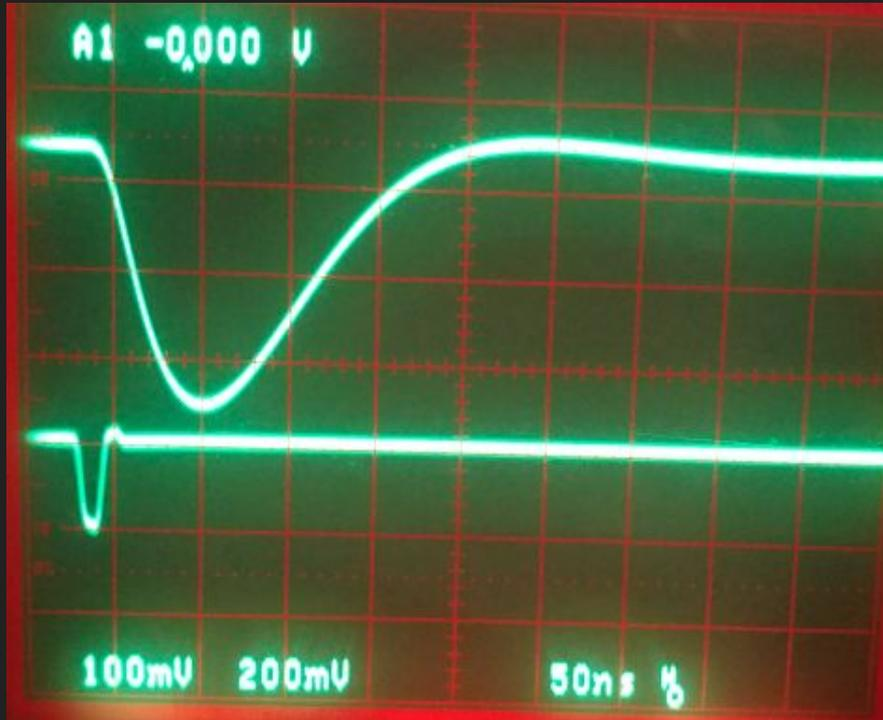
Distorted pulse due to saturated amplifier
