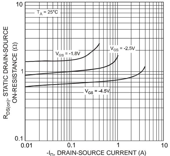
Fig. 6 Static Drain-Source On-Resistance vs. Drain-Source Current
