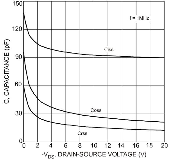
Fig. 10 Typical Capacitance
