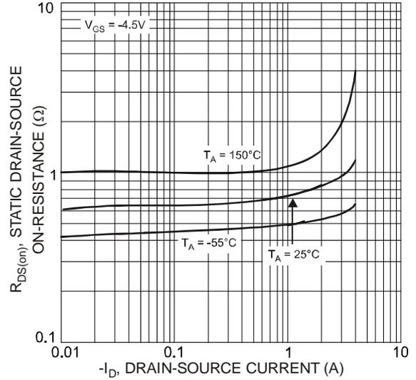
Fig. 4 Static Drain-Source On-Resistance vs. Drain Current
