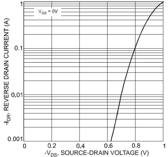
Fig. 8 Reverse Drain Current vs. Source-Drain Voltage
