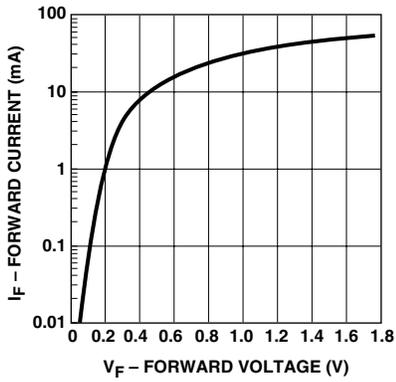
Figure 1. Typical Forward Current vs. Forward Voltage.
