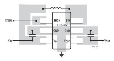
Figure 3. Recommended Component Placement
