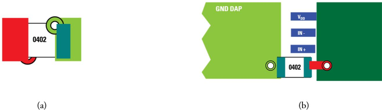
Figure 30. Typical Decoupling Capacitor Layouts
