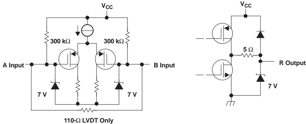
Figure 17. Receiver Equivalent Input and Output Schematic Diagrams
