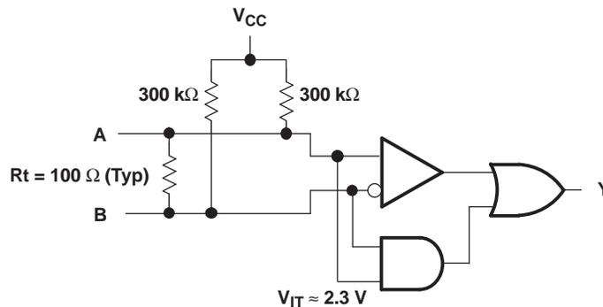
**Figure 16. Open-Circuit Fail-Safe of the LVDS Receiver**
