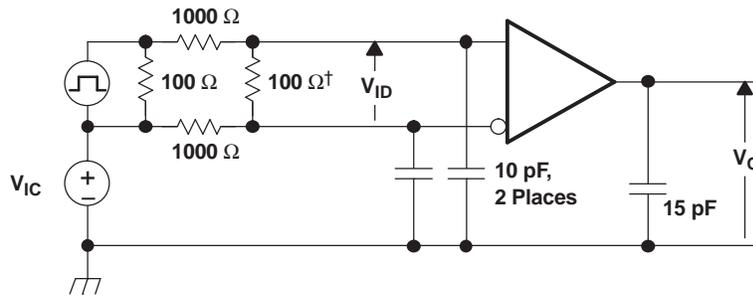
† Remove for testing LVDT device.
