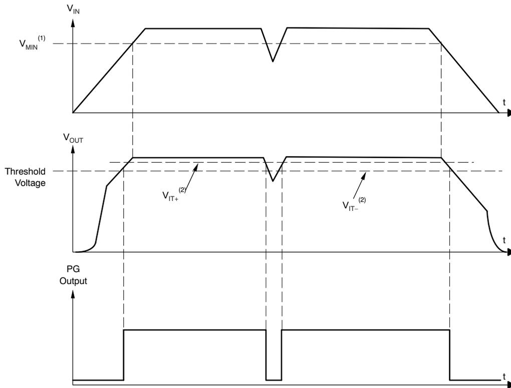
NOTES: (1)  $V_{MIN} = V_{OUT} + V_{DO}$ .
